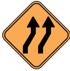
Dual Lane Realignment
